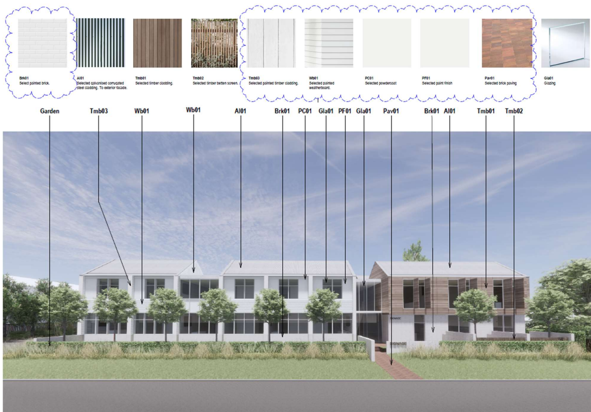
Figure 10: Extract from the materials and finishes plan for the accommodation building (H&E Architects, 2024)
